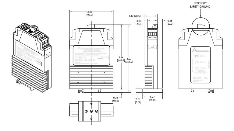
SMARTSafe™ is a trademark of Avtron Industrial Automation, Inc. Features and specifications subject to change without notice. Avtron standard warranty applies. All dimensions are in inches (mm).
