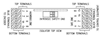
Vs = 12 TO 24 VOLTS DC Is = 850mA MAX., 300mA TYP.
