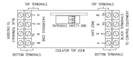
TYPICAL CABLE 500' (150M) MAX 18AWG, 4 Twisted Pair + Overall Shield BELDEN P/N 1064A OR AVTRON B37178 CUSTOMER EQUIPMENT PHASE DIFFERENTIAL · VŎLŤS B \*12-24 | Louts out GND GND ENCODER LINE DRIVER OPTION H OR 5. SEE INSTRUCTION \* MAX. SAFE AREA VOLTAGE Um = 30V Vs = 12-24 VDC Is = 850mA MAX 300mA TYP SHEETS FOR CONNECTOR OPTION PIN OUTS & PHASING HAZARDOUS AREA INTRINSIC SAFETY GND IN ACCORDANCE WITH SAFE AREA ZONE 1 GROUP IIC IEC/EN60079-14 & IEC/EN60079-25 ZONE 21 GROUP IIIC
