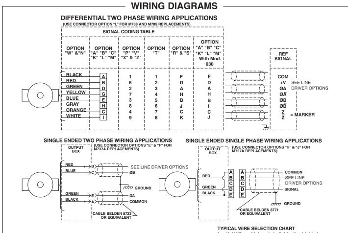
NOTES: Marker output for connector options "E" & "F" - Pin "D" Marker output for connector options "H" & "J" - Pin "C"
