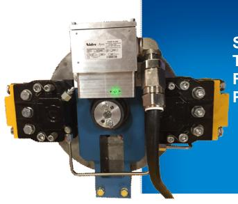
Severe Duty Encoder for TDS9/10/11 Mounting with Flameproof and Explosion Proof Ratings
